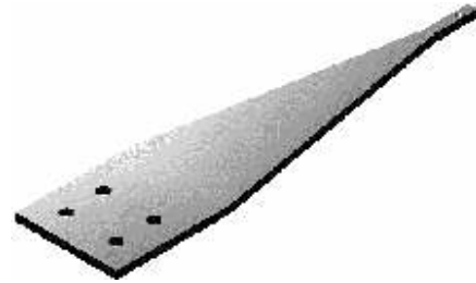
Figure 1. Constant Stress Beam.
