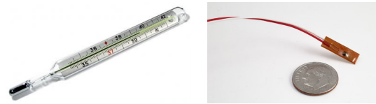
Figure 1-2. Mercury Thermometer (left) and Resistance Temperature Sensor (right)
